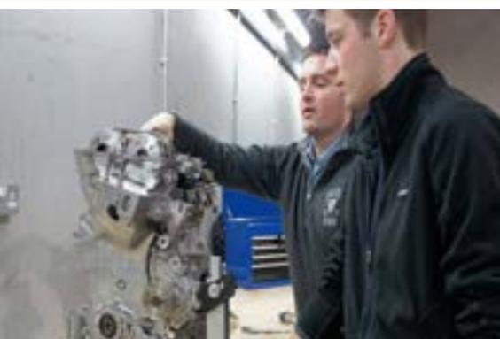
We have also taken delivery of 4 engine and gearbox stands which have allowed us access to the full disassembly of our 3 cylinder Hyundai engine. This has allowed us to complete essential engine inspections and complete routine repairs and servicing such as timing chain inspection/replacement.
